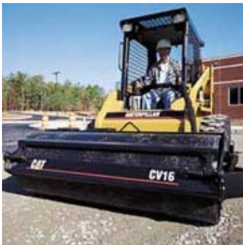
Skid Steer with Vibratory Drum
