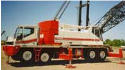
Lattice Truck Crane
